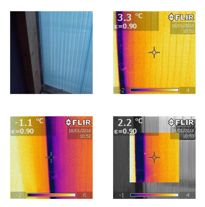
You notice how the temperature distribution on the inner side reflects the external situation with a significant difference (about 5 ° C) between the polycarbonate and the aluminum profile.
