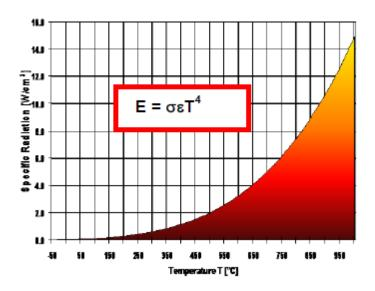
In reality, besides the temperature, the radiated energy depends linearly on the parameter emissivity, pure number included between 0 and 1 indicating substantially the efficiency of thermal radiation.
