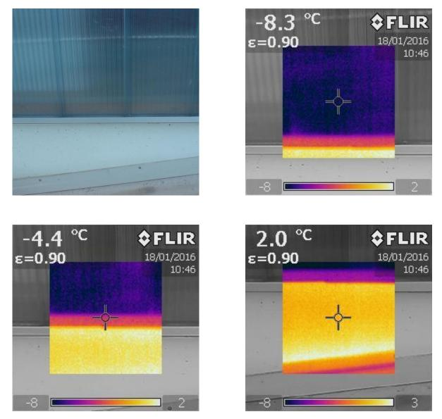
The outer side presents some significant temperature differences of the different materials: polycarbonate has a temperature of the external surface equal to -8.3  $^{\circ}$  C, the aluminum profiles without thermal break -4.4  $^{\circ}$  C, the concrete masonry 2.0  $^{\circ}$  C.
